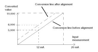
The alignment value is editable from a programming console, even if the program is in RUN mode. For each input channel, you can:
