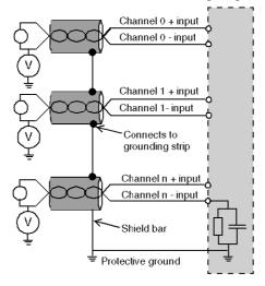
If the sensors are referenced in relation to the ground, this can return a remote ground potential to the terminal block. To help avoid this situation, follow these rules:
