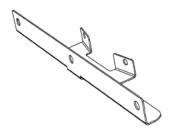
Screw foot to fan as shown Using the self drilling / tapping screws provided. (A pilot hole maybe required).
