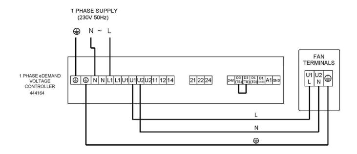
Fig. 6 ACQ10012D, ACQ12512D, ACQ15012D, ACQ16012D. Connected to an eDemand inverter
