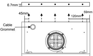
Figure 4: Screw locations for wall mounting
