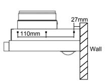
Figure 5: Screw locations for cupboard mounting
