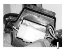
Figure 3: Placing the socket and plug in the connection box
