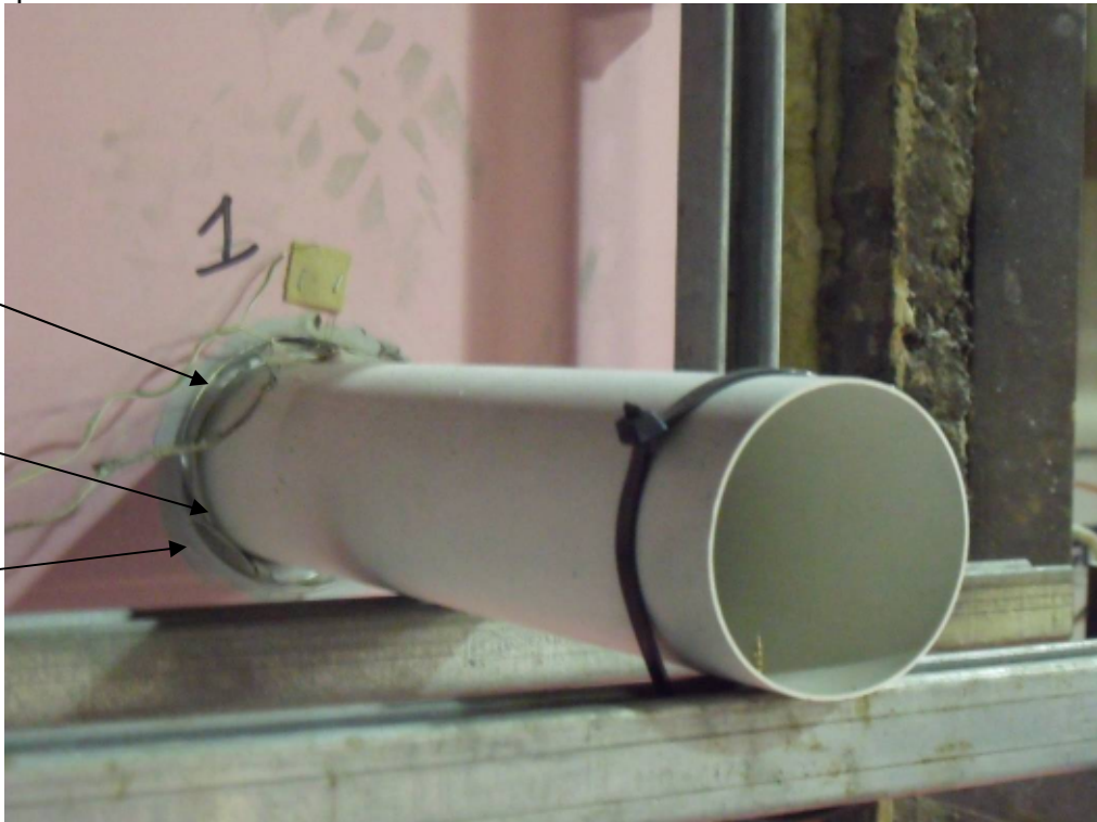
Unexposed face – Duct E support system and Tenmat steel sleeve with Tenmat vent duct wrap
