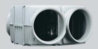
A 'stand alone' heat exchange module which will transfer up to 70% of the outgoing heat to incoming air. Polymeric construction with spigots to suit 200, 250 and 315mm  $\varnothing$  flexible ductwork.
