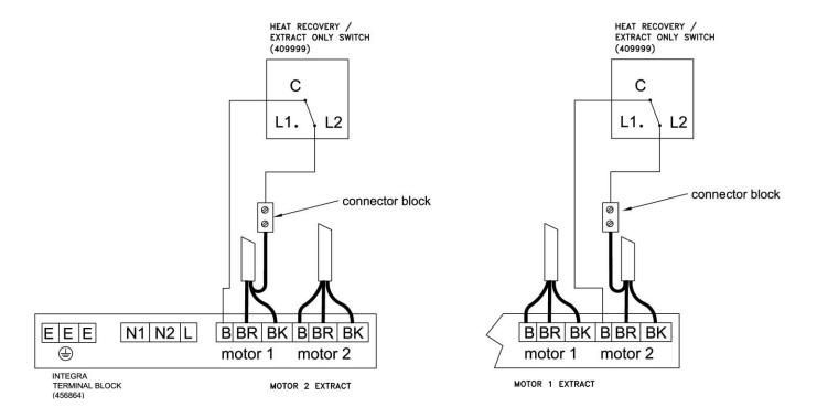
Where an extract only switch is to be used the blue wire for the **supply** motor needs to be connected to the switch as shown. The L, N1, N2 and E terminals should be connected as per the relevant Fig.2. After installation ensure that with the switch set to extract only that there is no supply airflow.
