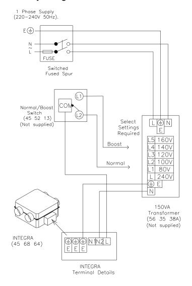
Fig.2d (Integra controlled via two sensors/switches and a 150VA transformer to give 3 running speeds).
