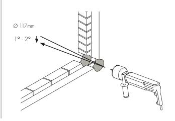
**Step 3**Measure hole and note length, if deeper than 25cm, go to step 5. If shorter than 25cm, trim the outer pipe's ears - go to steps 3 + 4.
