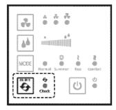
The light for filter maintenance lights up when selected period listed, (default 180 days). Change the air filter according to the instructions, see page 12. **Replacement Filters Ref:- 411158**
