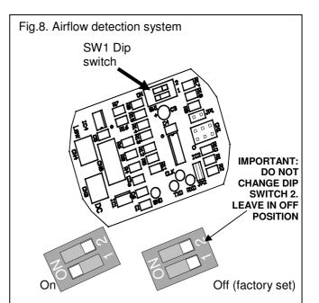
**Auto sensing mode** = Push switch (SW1) into the on position to turn on airflow detection system.
