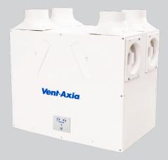
A wholehouse heat recovery system with up to 94% energy efficiency. An easily accessible heat recovery cube protected by two removable ISO 45% Coarse (G3) Filters. Two Lo-Carbon Energy Saving EC/DC fans ensure long life (typically over double the life of AC motors) and lowest possible energy use. Fully insulated construction with built-in condensation drain.
