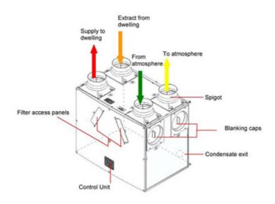
Figure 1: Kinetic Plus E (Front of Unit as supplied)
