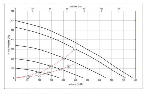
Note: Graph show 2 typical system curves with total unit input power in Watts.
