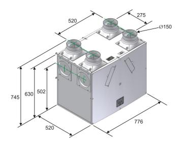
Figure 2: Kinetic Plus E Dimensions
