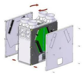
The arrow labels on the top edge of the Covers should be correctly matched to the arrow labels on the top of the Case.
