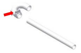
**6.** Fit pipe assembly into waste pipe and secure 90 deg elbow to condensate spigot with worm drive clip.
