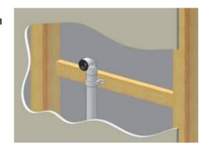
Fit the 180 degree bend supplied to a 22mm diameter x 280mm long condensate pipe with worm drive clip.
