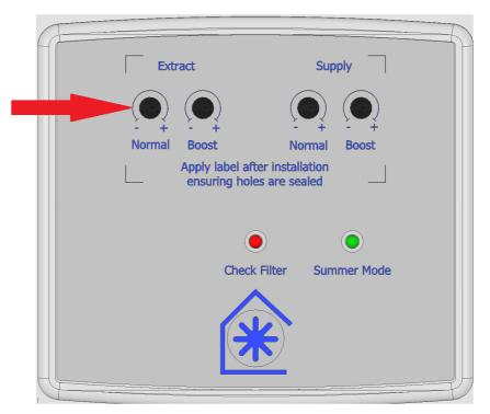
Figure 3: KINETIC PLUS E Controls
