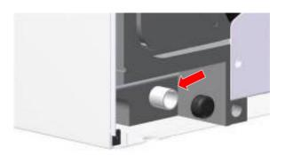
**3.** Fit the vertical condensate pipe and secure with worm drive clip
