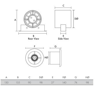
Internal/External Grille Dimensions 140x140mm Fan Transformer (W x H x D) 87 x 87 x 33
