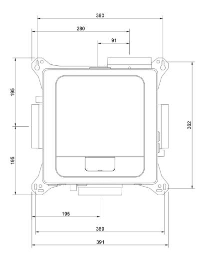
i. Base mounted Installation with ducting radiating out horizontally.
