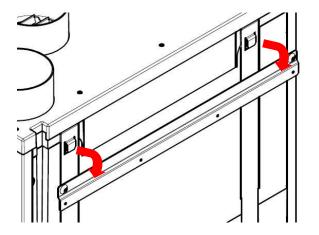
**Step 4:** Make sure the unit is level or leaning slightly backwards; this is to ensure the condensate drain functions correctly.
