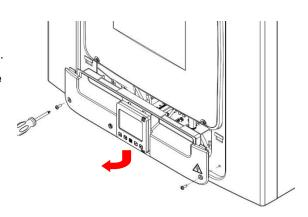
**Step 3:** Push the locking tab away from the printed circuit board and slide it outwards to access the terminals
