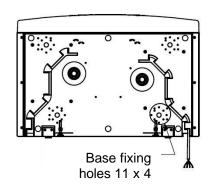
**Step 2**: Mount your chosen foot type to the underside of the unit using appropriate fixings.
