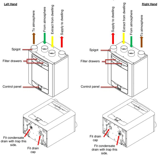
Figure 1: MVHR with Left-Hand and Right-Hand spigot configuration.
