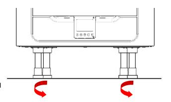
It is recommended that where possible, the wall bracket is used in conjunction with any floor mount solution to prevent the unit from tipping.
