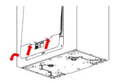
**Step 2:** Remove the inner door by undoing the 4 retaining screws.
