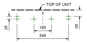
**Step 2:** Attach the wall bracket, using appropriate fixings.
