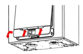
**Step 2:** Remove the two screws on either side of the access panel. Lift the panel outwards from the bottom edge to remove.
