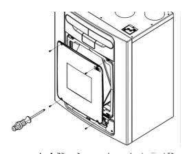
**Step 3:** Slide the heat exchanger out from the unit. (If cell is stiff to pull out of unit, pull cell strap from top, then from the bottom).
