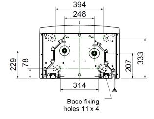
**Step 2**: Mount the board to the underside of the unit using appropriate fixings.
