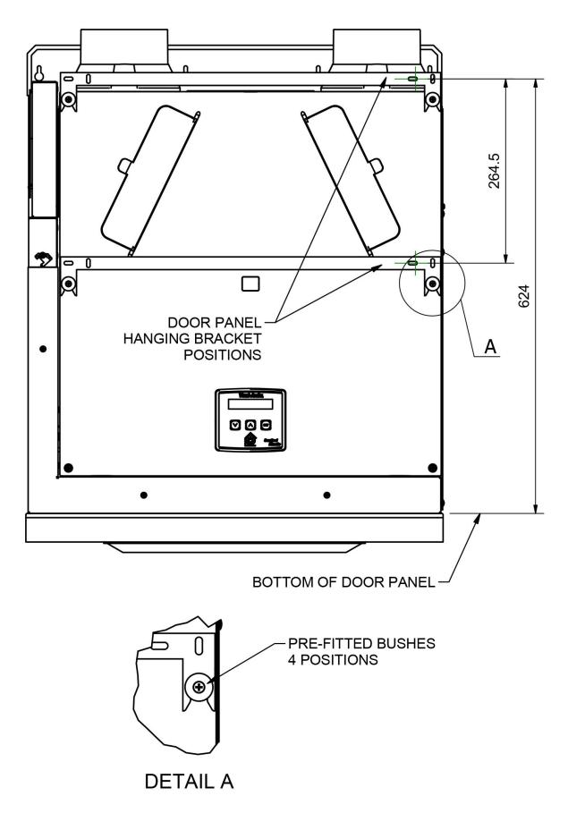
Figure 8: Door Panel Hanging Bracket Positions
