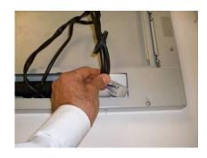
Figure 10: Insert cable opposite direction
