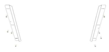
**Stage 2:** Place each of the bolts into position and **do not** fully tighten. Leave approximately "a half turn" loose on each of the fixings. This will allow each bracket to be moveable until final fitting of the unit and makes any adjustments easier while installing the unit in position.
