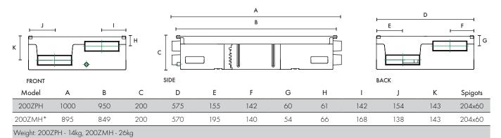
\*Galvanized steel outer case construction
