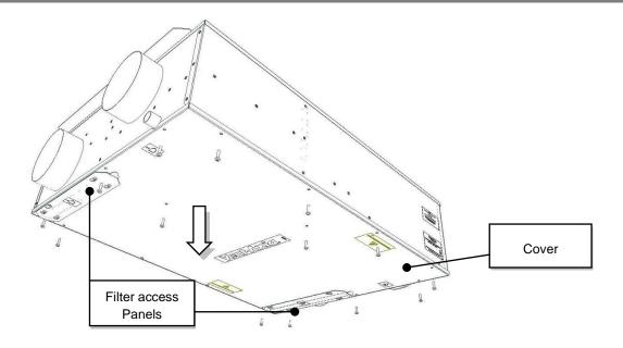
Stage 1: Isolate the mains power supply and remove the Filter access Panels and Filters. Undo the securing screws and remove the Cover .
