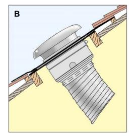
The illustration shows a T-Series roof model fitted with a direct mount spigot and flexible ducting.
