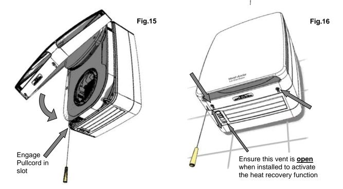
14) The Tempra unit is also fitted with a "manual summer setting" which allows the unit to be set to extract only, helping to prevent a dwelling becoming too warm in hot summer conditions. When first installed this shutter/vent should be **open**. Fig.16 To activate the summer setting it should be shut.
