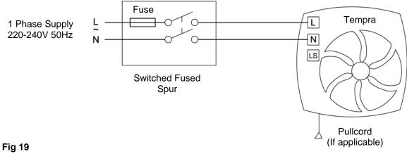
Continuous trickle (6l/s or 9l/s) with switch live boost facility.
