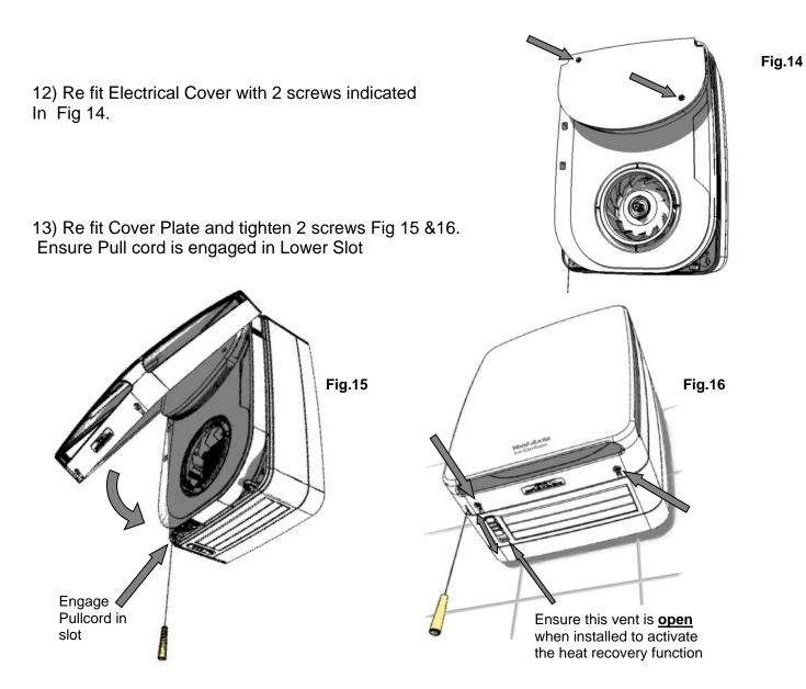
14) The Tempra unit is also fitted with a "manual summer setting" which allows the unit to be set to extract only, helping to prevent a dwelling becoming too warm in hot summer conditions. When first installed this shutter/vent should be **open**. Fig.16 To activate the summer setting it should be shut.
