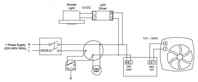
Fig 2. LuminAir Kit T (Ref. No 453413A)
