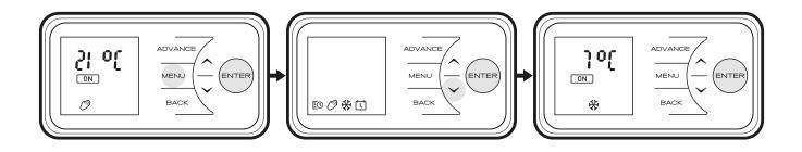
Standby - Select standby to switch off the heating element. Heat will not be provided.
