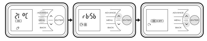
**Open Window** - The heater comes with a feature that will detect if a window is open and heat is being lost, so the heater will enter a reduced-power mode instead of using unnecessary energy. Open Window detection is activated by default. To activate/deactivate this feature:
