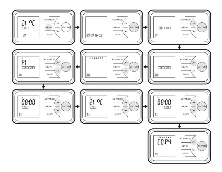
Once P1-P4 heating programmes have been set, **COPY** will flash on the screen. To copy newly programmed P1-P4 heating programmes to other days press the **Enter** button.
