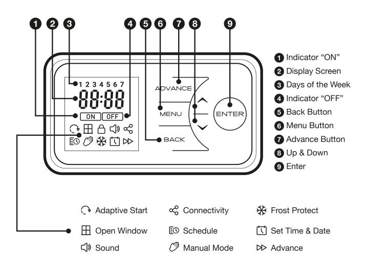
The heater is fitted with an adjustable thermostat enabling the room temperature to be controlled. The minimum room temperature is 7°C. The maximum temperature is set to 26°C by default, however, this can be increased to 32°C if required. A temperature of 21°C would be comfortable for most people.
