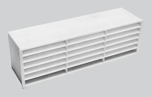
Available in five colours, this low resistance air brick has been designed to comply with the latest Building Regulations Approved Document F, which requires a ventilation outlet to achieve a minimum of 90% of the cross sectional area of the ductwork.
