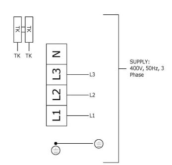
Note: A trial connection should be made in order to check that the direction of fan rotation is correct. If incorrect, interchange any two phases of the three phase supply.
