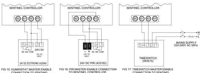
FIG 15: HUMIDISTAT MASTER ENABLE CONNECTION TO SENTINEL CONTROLLER (NOTE! ENSURE LINK 61-62 IS REMOVED)
