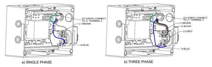
FIG 8: CONTROLLER MAINS SUPPLY CONNECTIONS
