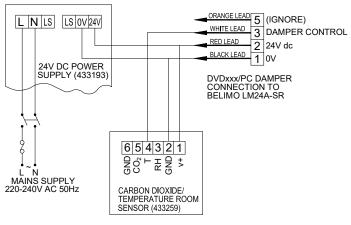
FIG 28C: TEMPERATURE ROOM SENSOR CONNECTION TO PROPORTIONAL DAMPER
