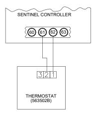
FIG 18: THERMOSTAT MASTER ENABLE CONNECTION TO SENTINEL CONTROLLER (NOTE! ENSURE LINK 61-62 IS REMOVED)
