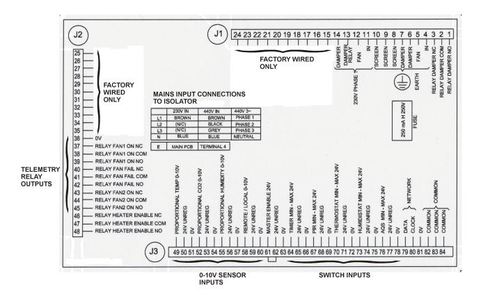
Fig.1 Controller Connections Layout
