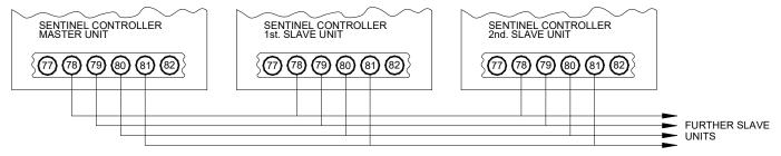
FIG 24: MASTER-SLAVE NETWORK CONNECTIONS
