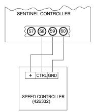
FIG 21: REMOTE SPEED CONTROL CONNECTION TO SENTINEL CONTROLLER This nominally provides for air extraction but can also control a balanced intake – extract system if suitably configured with a Sentinel slave unit.
