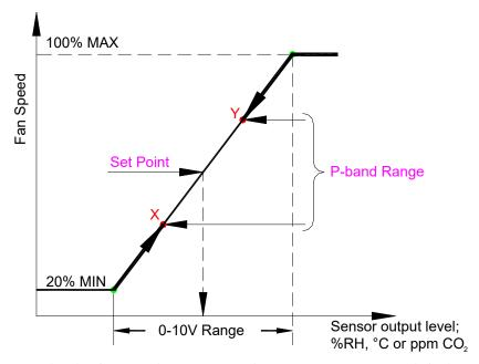
If, for example, the fan speeds are 20% and 100% (Note! Factory defaults are 20% and 80%), and the P-band range is equivalent to, say, X and Y, then point X becomes the 20% fan speed and point Y becomes 100%. It can be seen that if the P-band is set too narrowly, the fan speed response becomes coarse.
