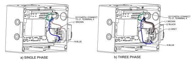
FIG 8: CONTROLLER MAINS SUPPLY CONNECTIONS
