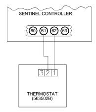
FIG 18: THERMOSTAT MASTER ENABLE CONNECTION TO SENTINEL CONTROLLER (NOTE! ENSURE LINK 61-62 IS REMOVED)
