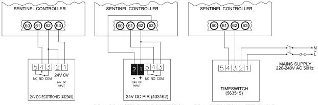
FIG 15: HUMIDISTAT MASTER ENABLE CONNECTION TO SENTINEL CONTROLLER (NOTE! ENSURE LINK 61-62 IS REMOVED)
