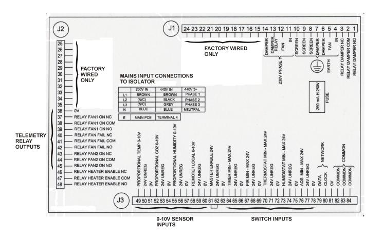
Fig.1 Controller Connections Layout
