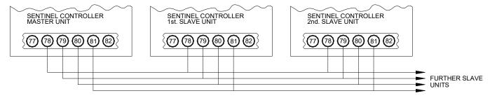
FIG 24: MASTER-SLAVE NETWORK CONNECTIONS
