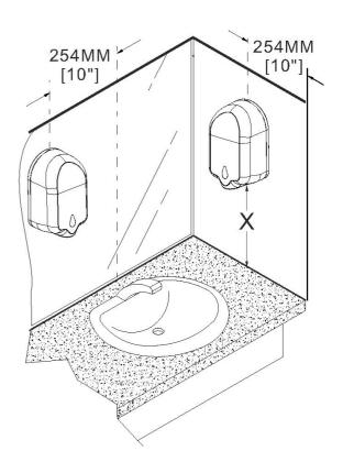
"X" Distance [ Minimum ]: Normal Counter Top: > 200 MM Stainless Steel Counter Top: >300 MM
