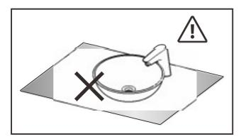
It is recommended to avoid installing the dispenser near high reflective objects (mirror, stainless steel washbasins, etc.) in order to avoid faulty function of the presence sensor.
