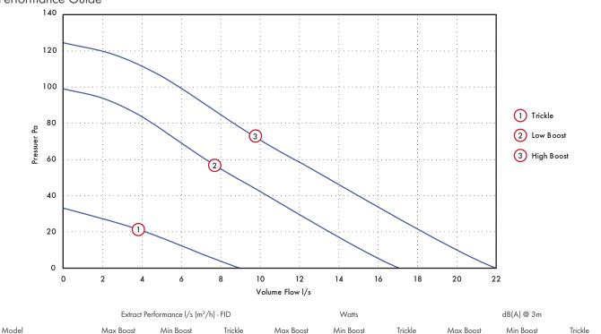
Model Min Boost Trickle Trickle Min Boost Max Boost Min Boost Max Boost Solo Plus P/T/HT/TM 9 (32) 10.9 6.3 11.5 22 (80) 17 (61) 17.1 34.5 24
