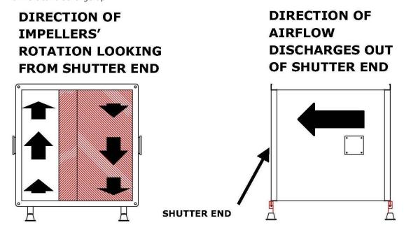
The TDF600 can only be mounted with the fans top and bottom (and the shutter shafts horizontal), discharging air horizontally.
