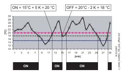
If the ambient temperature is higher than the set operating point, the cooling remains switched on. If the ambient temperature falls below the set operating point of the cooling by 2 K (Kelvin), it is switched off. I.e., the OFF point is situated at the hysteresis value under the ON point.
