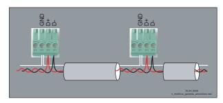
general example for Modbus device connection
