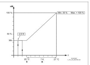
Minimum speed cut off (idealized principle diagram)
