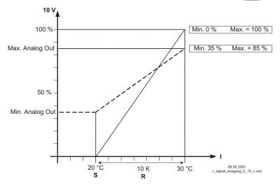
Example: Setpoint ventilation 25.0°C, Offset -5.0 K, Pband 10.0 K
