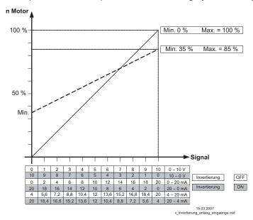
nM Motor speed Si Signal OFF Inverting = OFF ON Inverting = ON
