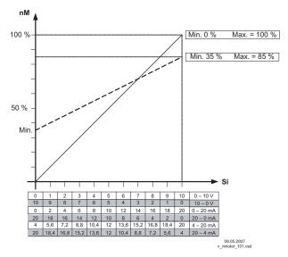
nM Motor speed Si Signal
