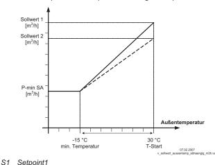
An outside temperature compensation can be activated (sensor connection "E2" to "Analog In 2") when being operated as a air volume regulation device.
