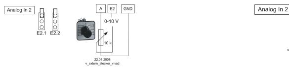
External Setpoint via external signal instead of "Setpoint 1". The "external Setpoint" function must be activated in base setup 1E for "E2 function". The active external Setpoint value is displayed in the "info" menu group.
