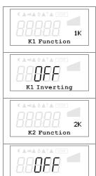
Various functions can be allocated to the relay outputs "K1" and "K2". In case of the same function allocation for "K1" and "K2", these work parallel.
