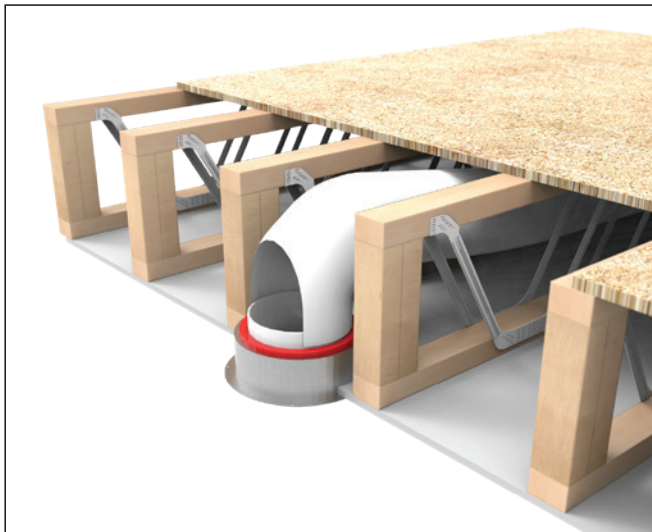
Ceiling Fan Firestop expands when exposed to heat.
