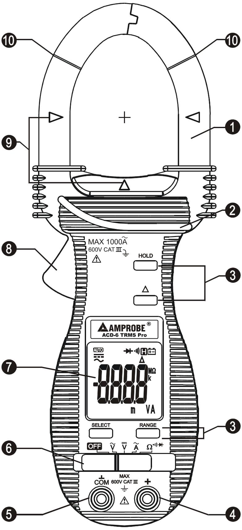
1) Transformer Clamp Jaw for AC current magnetic field pick up
