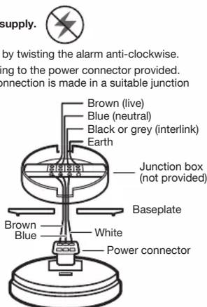
If desired, the alarm can be interconnected with up to 11 other smoke, heat or carbon monoxide alarms from the FireAngel range via the 'I' connector. (See Optional Interconnecting Feature).
