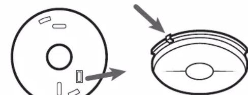
To enable removal of the alarm, withdraw the locking plug with a pair of pliers.
