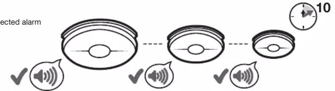
On an interconnected network, only the alarm that senses the fire will sound and flash its LED. Other connected alarms will sound a warning but will not flash their LED. Do not connect more than 12 devices.
