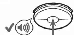
Your alarm requires 1 x 9V (PP3) battery. Under normal use, the battery should last approximately one year. Use of a battery other than those recommended here may have a detrimental effect on the alarm:
