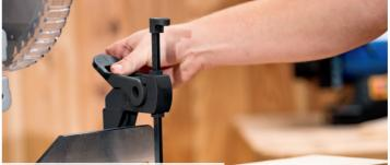
Work piece clamp with quick-release lock.
