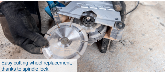
Additional guide wheels on the sides allow precise guidance of the tool.
