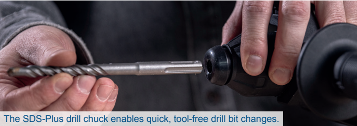
The SDS-Plus drill chuck enables quick, tool-free drill bit changes.
