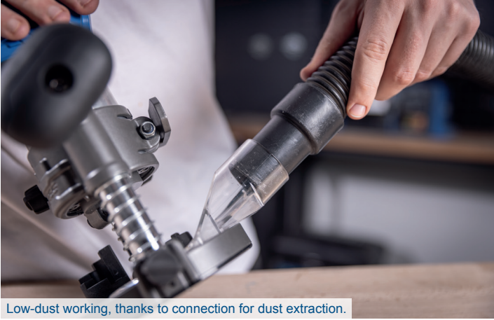
Low-dust working, thanks to connection for dust extraction.
