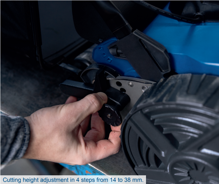
Cutting height adjustment in 4 steps from 14 to 38 mm.
