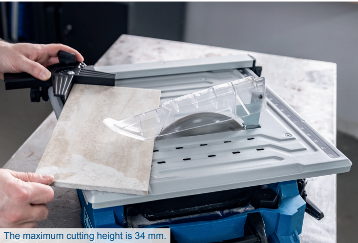
The maximum cutting height is 34 mm.
