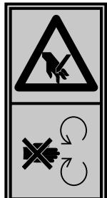
DANGER – Rotating blades. Keep hands and feet out of openings while machine is running!
