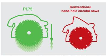
The advantage compared with conventional hand-held circular saws is the plunge function. Using this function, specific demands that require plunging the saw blade into the material can be implemented without problems.
