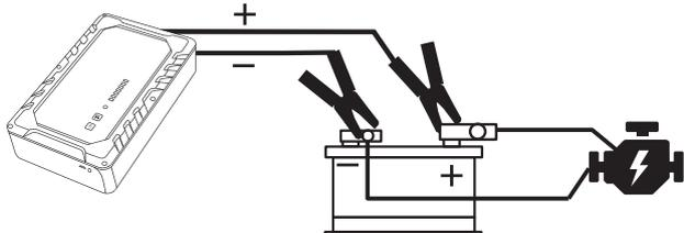
Connect the red clamp (+) to the battery's (+) terminal.
