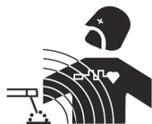
The electric current flowing through any conductor causes electrical and magnetic fields (EMF). The welding current generates an EMF around the welding circuit and the welding equipment.
