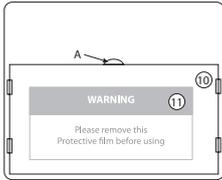
The internal protection screen (10) is removable by sliding it down by placing a finger on (A). When changing the screen, make sure you remove the protective screen (11)
