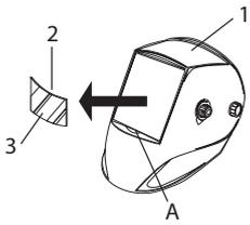
The outer protection screen (2) can be removed by placing a finger under the screen on (A) of the helmet (1). When changing the screen, make sure that the protective film (3) has been removed. This film must be removed only when the protection screen is in position in the helmet.
