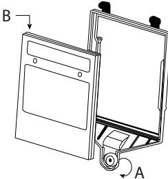
1. Unscrew the filter retainer (A)
