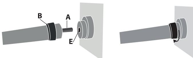
Insert the torch's connector (A) in the female compartment (E) and screw the B part. Be careful to tighten the torch.
