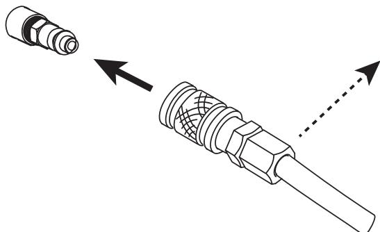
Connecting the gas supply to the current source by means of an inert gas pipe of an internal diameter of 9.5 mm and a quick connect coupler.
