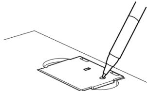
The red LED next to the learn in button will flash briefly then light up for approximately five seconds to show that it is ready to receive the "learn in" signal. During the next 5 seconds you will need to briefly press the test button on Alarm 1 to wirelessly interlink the two alarms.
